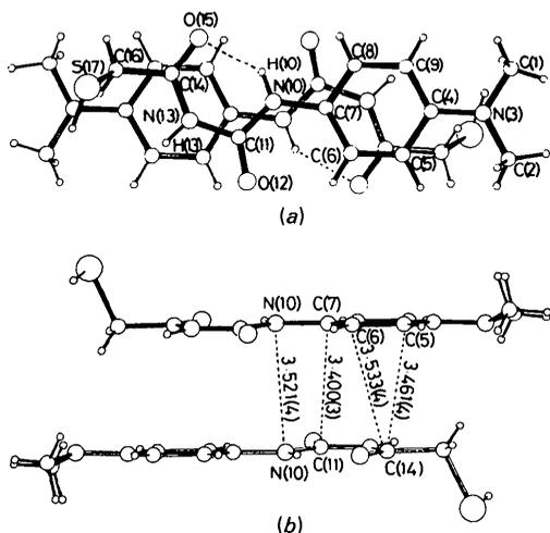
Fig. 2. The overlapping mode of the two molecules around the inversion center ( $\frac{1}{2}, \frac{1}{2}, \frac{1}{2}$ ): (a) projection along the normal to the mean plane of the acylurea moiety and (b) side view. Several contacts (Å) are given.
